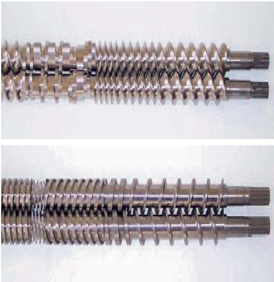
FIGURE 4. Twin screw design examples: intermeshing co-rotating twin-screw (top), and intermeshing counter-rotating twin-screw (Burns et al.). (Courtesy of American Leistritz Co., Somerville, NJ) (bottom).
